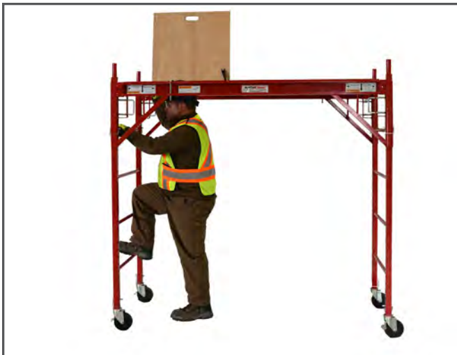
Climbing end frame within the Scaffold through Hatch - Safe working load 125kg (275lbs) Safety factor 2:1
