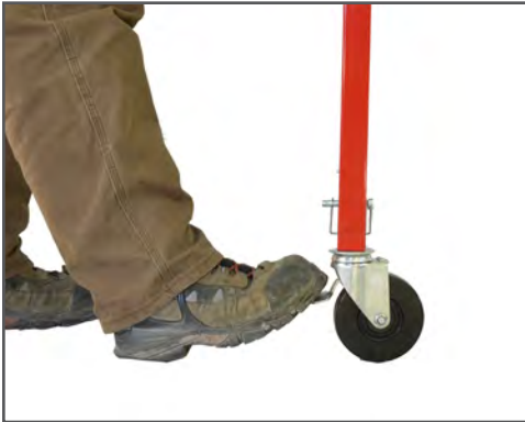
1. Prior to installing outriggers, confirm casters are in the locked position.
