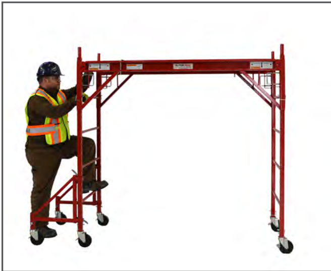
Climbing end frame within end outriggers - Safe working load 125kg (275lbs) Safety Factor 2:1
